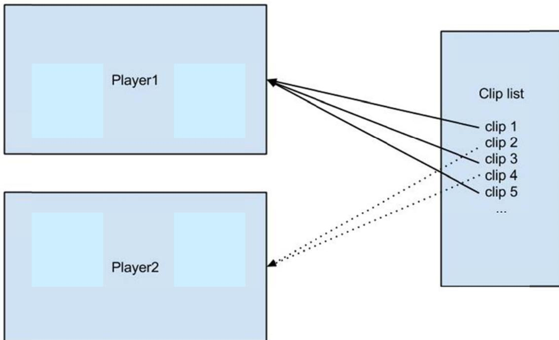
**Figure 4-8: How preloader works**
