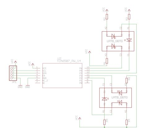
Figure 4.1: Schematic of the LED module
