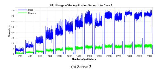
Figure 2.15: CPU usage of the application servers for case 2
