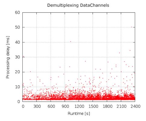
Figure 3.17: Processing delay of demultiplexing DataChannels
