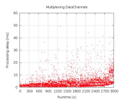
Figure 3.13: Processing delay of multiplexing DataChannels
