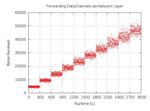
Figure 3.10: Received throughput of network layer. Sent throughput was the same.
