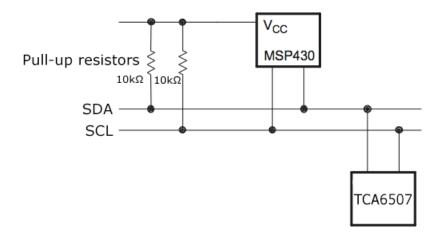
Figure 4.3: General overview of  $I^2C$  bus. SCL and SDA are pulled up with resistors. The LED module does not have these resistors as Earl already has these resistors.
