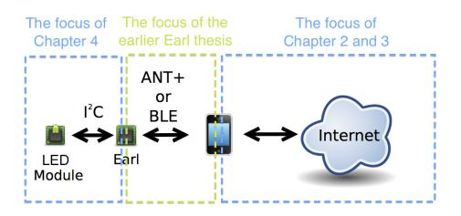
Figure 1.1: The relationships between LED module, Earl, mobile phone, and Internet for this thesis project. This figure also illustrates the relationship of this project to the earlier Earl thesis project [6]
