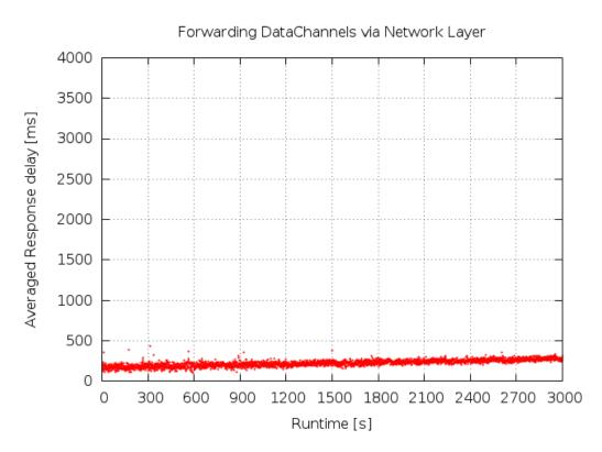
Figure 3.8: One-way delay of network layer
