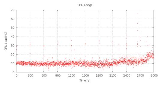
Figure 3.15: CPU usage of multiplexing DataChannels
