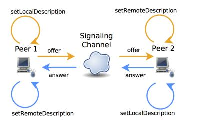
Figure 3.7: SDP flow in WebRTC
