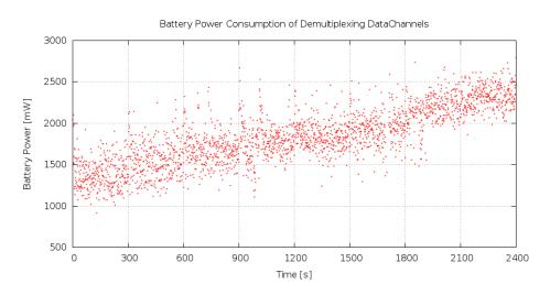
Figure 3.20: Battery power consumption of demultiplexing DataChannels
