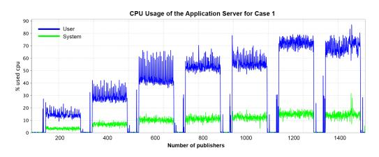
Figure 2.14: CPU usage of the application server for case 1
