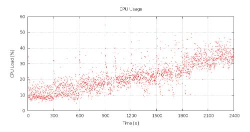
Figure 3.19: CPU usage of demultiplexing DataChannels
