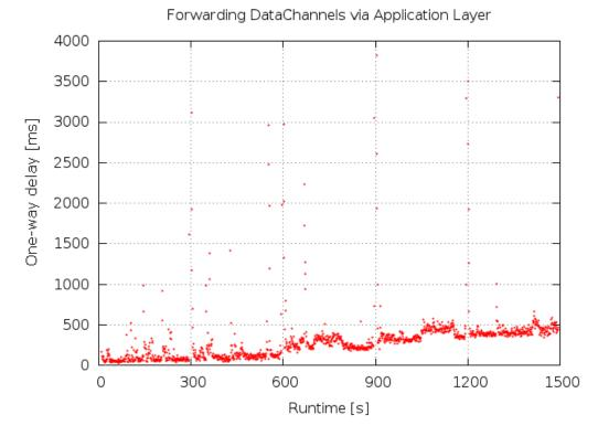
Figure 3.9: One-way delay of application layer
