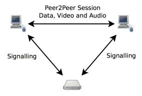
Figure 3.1: Overview of the WebRTC architecture
