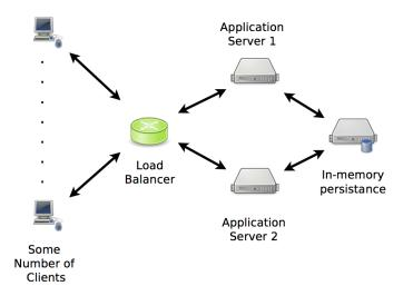
Figure 2.1: Overall view of the architecture for the WebSocket tests
