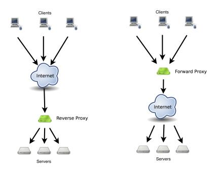
Figure 2.4: Forward proxy acting on behalf of the client. Reverse proxy acting on behalf of server.
