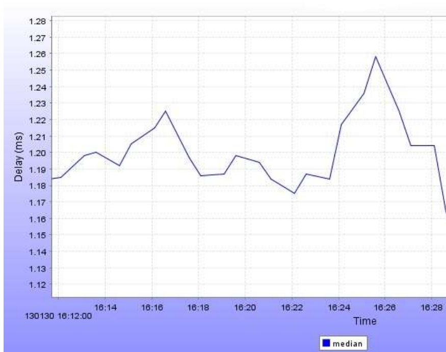
Figure 5-11: Network delay measured by “Accedian” probes for 10 minutes
