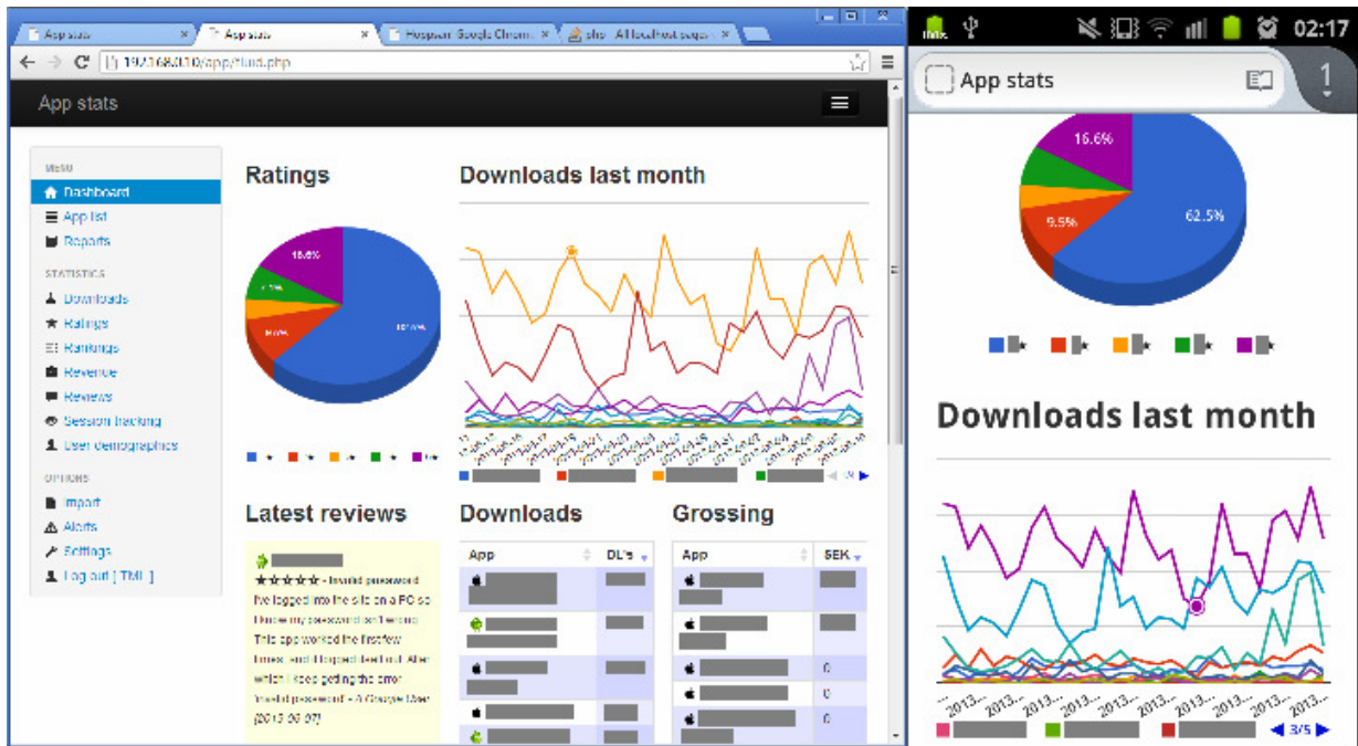
Figure 9-3 – Responsive design with Twitter Bootstrap (laptop version on the left and smartphone version on the right)
