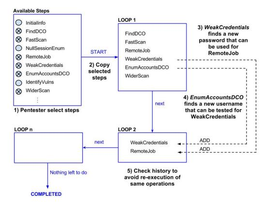
Figure 6.1: Example of an automated penetration test.
