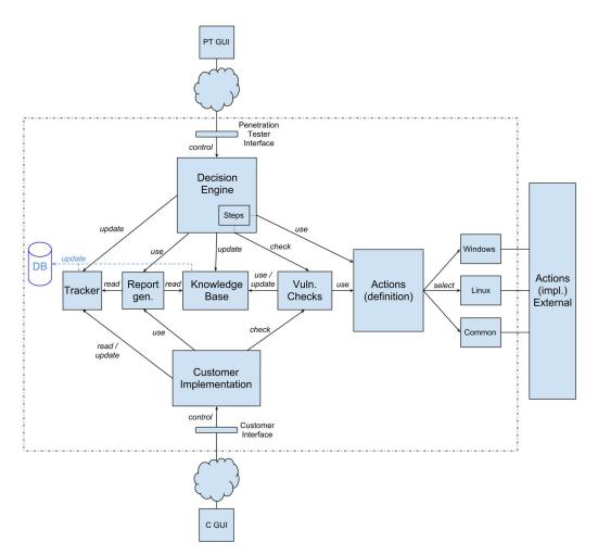
Figure 5.1: Architecture of the proposed automated penetration testing tool.
