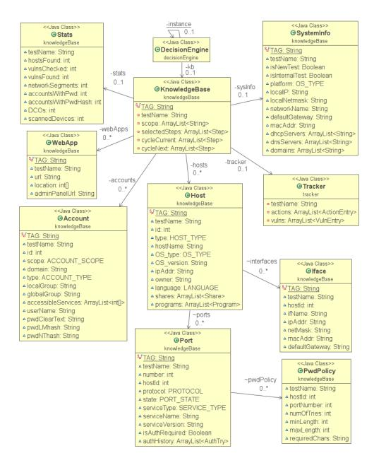
Figure 5.2: UML class diagram of the main classes in the knowledge base.
