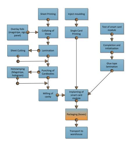
Figure 1.2: Card body Manufacturing Flow Chart [9]
