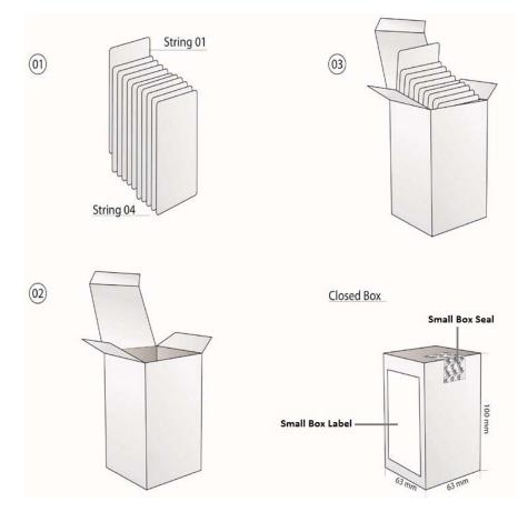
Figure 2.17: Small Box Scratch/Bank card Packaging
