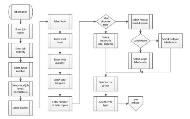
Figure 4.10: Flow chart: Job initial setup
