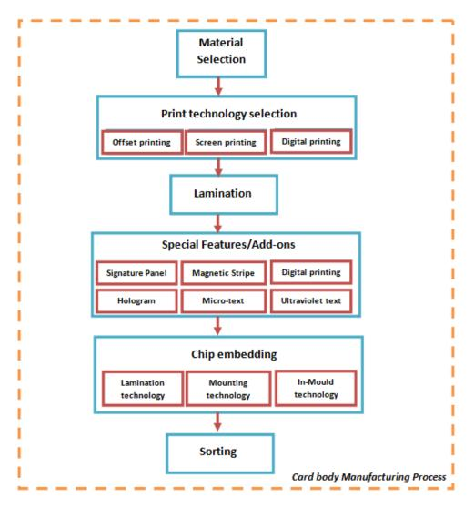
Figure 2.6: Card Body Manufacturing Process
