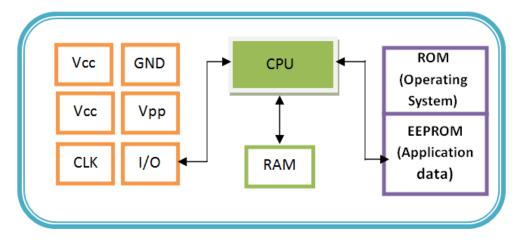
Figure 2.4: Architectural view of a microprocessor card [11]
