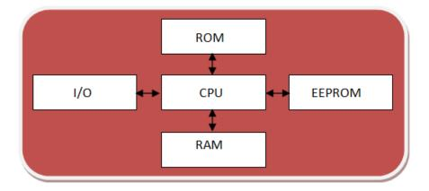
Figure 2.1: Smart card Architecture [36]
