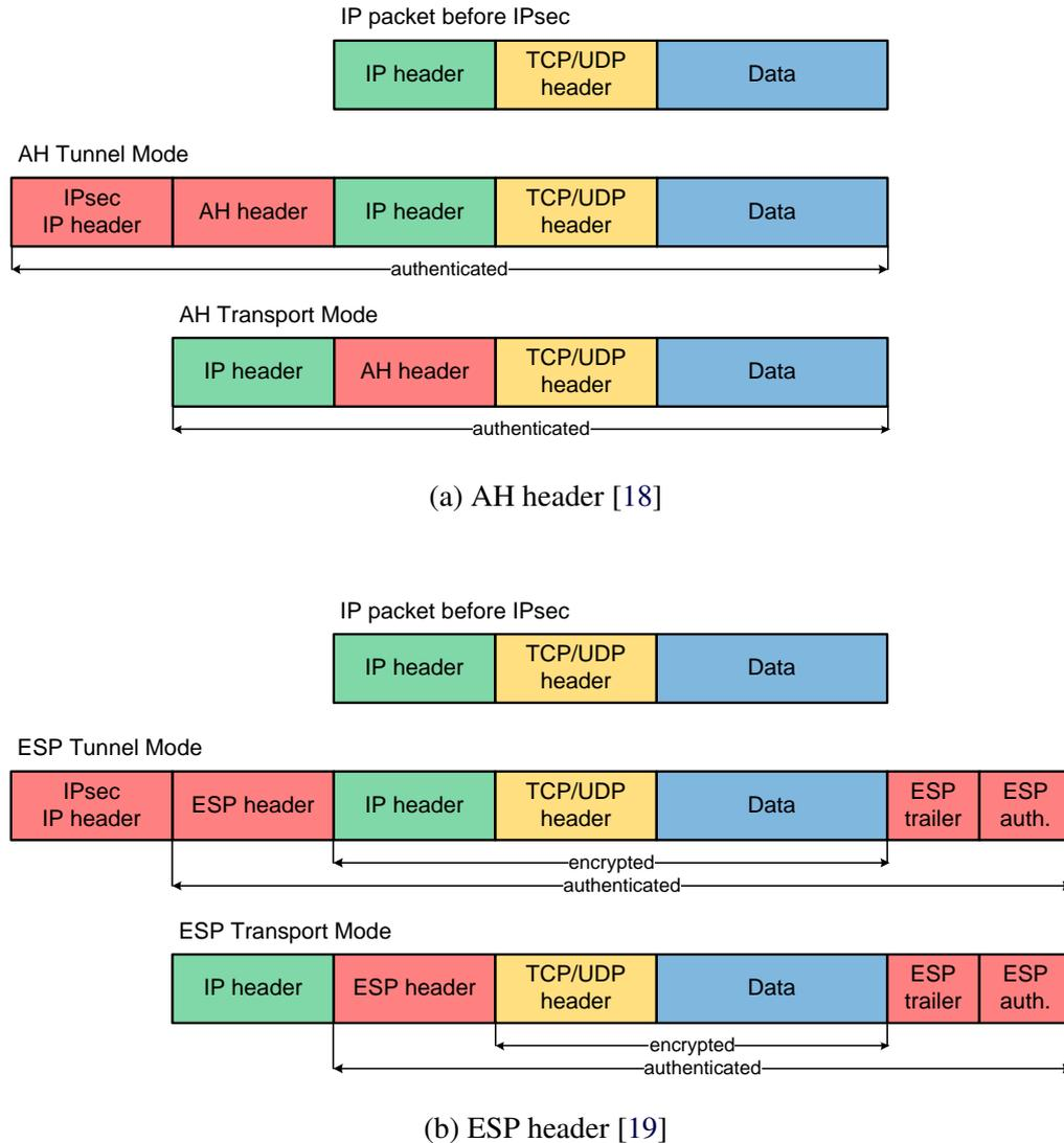
Figure 2.2: IPsec headers for tunnel and transport modes of operation
