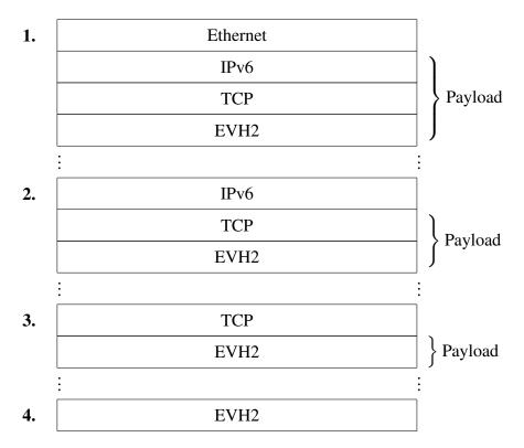
Figure 3.3: Encapsulation of a EVH2 packet
