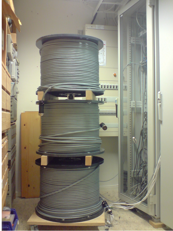
Figure 4.5.: 1,500 metres of a copper loop binder containing 24 twisted pairs
