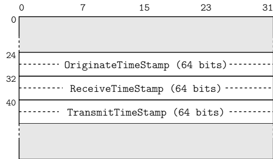
Figure 4.4: NTP packet header. Relevant fields for the synchronization procedure are shown highlighted.
