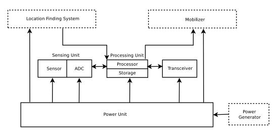
As shown in Figure 2.2, a sensor is composed of four main units [11]: a sensing
