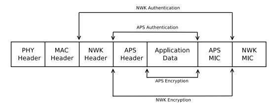
Figure 3.10: Authentication and encryption in ZigBee packets.
