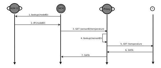
Figure 3.2: Flow of communications between MCN and a single sensor(s) that returns the temperature that it has measured locally.
