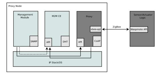
Figure 4.3: A prototype of the DHT-based M2M system, where a proxy is used to make WPAN nodes globally addressable and accessible from a 3G WWAN.
