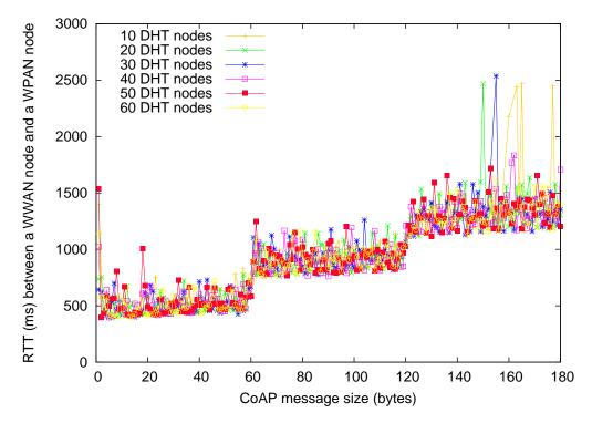
Figure 5.4: RTT is affected more significantly by the size of CoAP messages rather than the number of DHT nodes, when the majority of DHT nodes are virtual nodes residing on a single PC.
