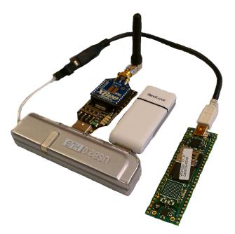
Figure 4.2: The hardware of the proxy prototype, where a Libelium Waspmote Gateway and a 3G dongle are connected to a Gumstix Overo Earth through a USB hub.
