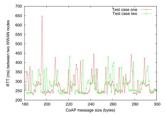
Figure 5.5: RTT between two WWAN nodes is not significantly influenced by CoAP message size, when CoAP messages are between 180 and 300 bytes.
