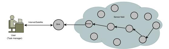
Figure 2.1: A multi-hop wireless sensor network.
