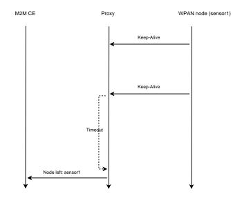
Figure 3.8: The "eagle" scheme in which WPAN nodes actively send keepalive messages to the proxy.
