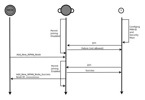
Figure 3.6: Node joining a ZigBee network.
