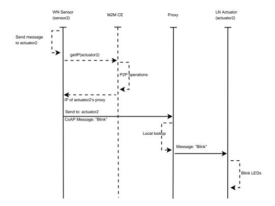
Figure 5.2: A sample scenario implemented in our prototype, where a WWAN sensor sends message to a local WPAN actuator.
