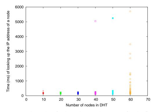
Figure 5.3: The number of nodes in the DHT does not significantly affect node lookup time, but he stability of node looking up decreases as the number of DHT nodes increases.
