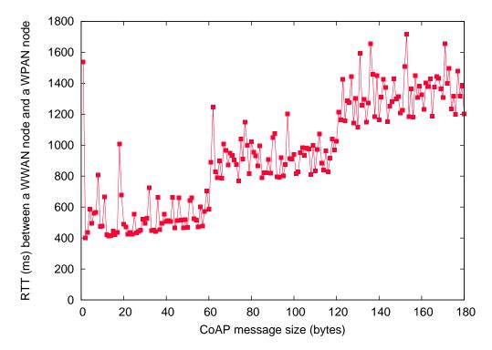
Figure 5.6: RTT is affected by the size of CoAP messages when the system has 50 DHT nodes (48 of which are virtual nodes residing on a single PC).
