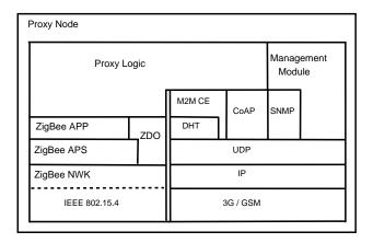
Figure 3.4: Protocol stack of the proxy node.
