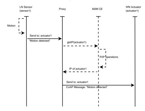
Figure 5.1: A sample scenario implemented in our prototype, where a local WPAN sensor sends message to a WWAN actuator.
