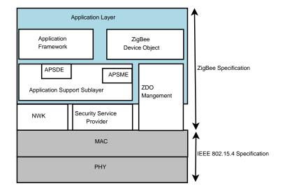
Figure 2.4: ZigBee stack architecture.
