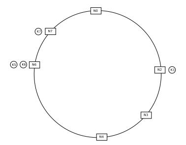
Figure 2.5: Illustration of a Chord ring.
