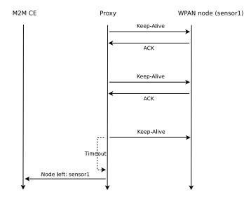
Figure 3.7: The "eagle" scheme in which the proxy polls WPAN nodes.
