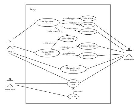
Figure 3.5: The UML use case diagram of the proxy.
