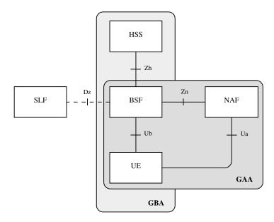
Figure 2.10: Network Elements for Bootstrapping with GBA and GAA
