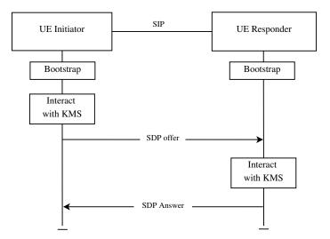
Figure 3.1: KMS Based Solution for Media Plane Security [4]
