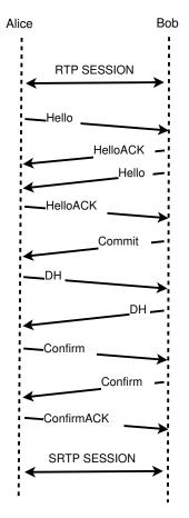
Figure 2.8: ZRTP Call Flow Example
