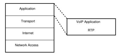
Figure 4.1: VoIP Application in TCP/IP Layer
