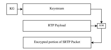
Figure 2.4: Default SRTP Encryption Process [1]
