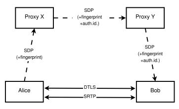
Figure 2.7: DTLS Message Exchange in SIP Trapezoid
