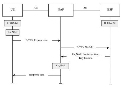
Figure 2.12: Bootstrapping Usage Process
