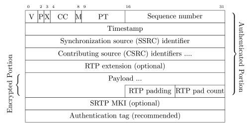
Figure 2.3: SRTP Packet Format [1]
