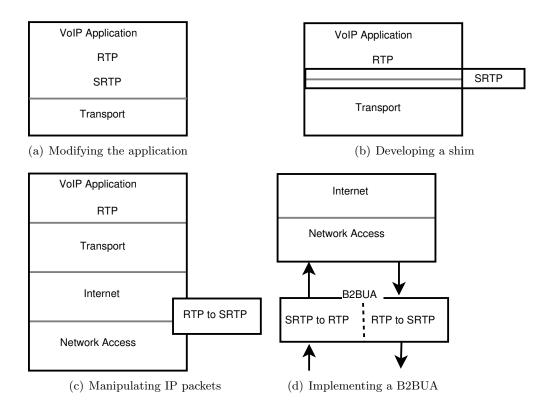
Figure 4.2: Alternative Approaches for Media Protection in Handset
