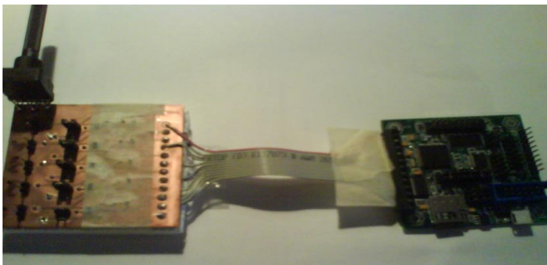
Figure 16 Sensor driving circuit and data acquisition board installation
