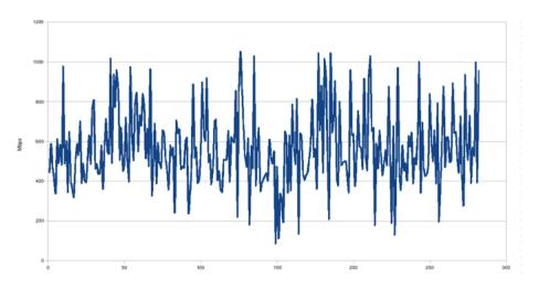
Figure 4.2: TCP bandwidth between two m1.small instances in Amazon EC2 (Source: [46])
