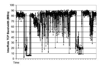
Figure 4.1: TCP bandwidth between two small instances in Windows Azure (Source: [39])
