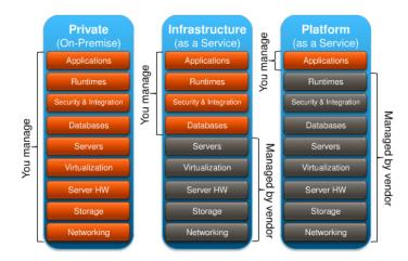
Figure 2.2: Server stack comparison between on-premise infrastructure, IaaS, and PaaS.
