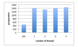
Figure 3.8: Iozone write test (time)
