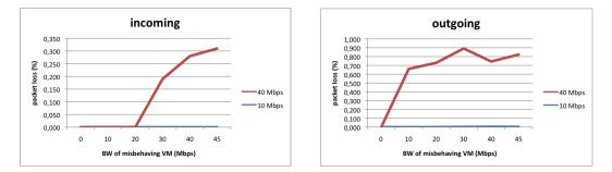
Figure 3.15: Packet loss stress test results
