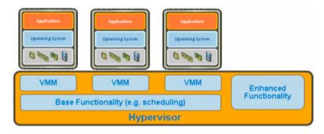
Figure 2.3: Diagram of an hypervisor virtualization layer with 3 VMMs running
