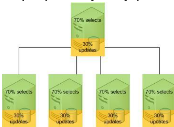
Figure 5 - Replicating a server that spends 30% on updating the database will only add 70% of the potential capacity in every new server.
