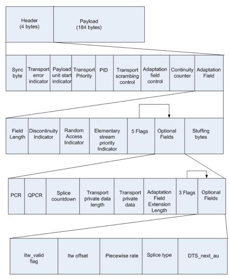
Figure 2.3: Overall Transport Stream, adapted from [18]
