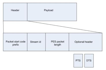
Figure 2.4: PES Packet Header, adapted from [19]
