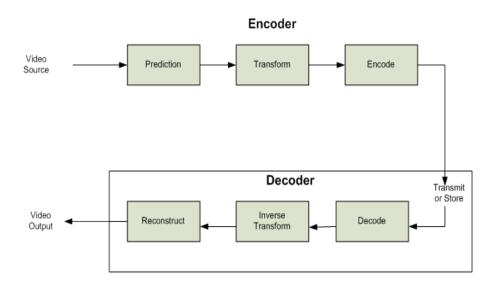
Figure 2.2: H.264 video encoding and decoding process, adapted from [13]
