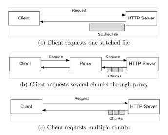
Figure 5.3: (a) Client requests one stitched file from the content server directly; (b) Client requests several chunks from the content server through the proxy streaming server; and (c) Client requests several chunks directly from the content server
