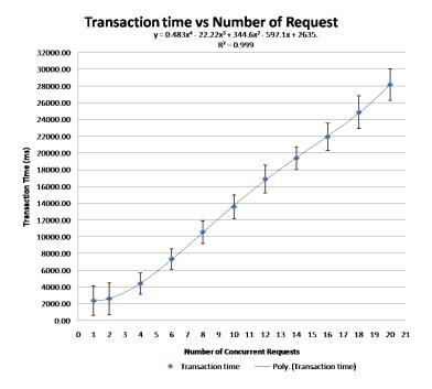
Figure 5.5: Transaction time vs number of concurrent requests - client requests several chunks directly from the content server
