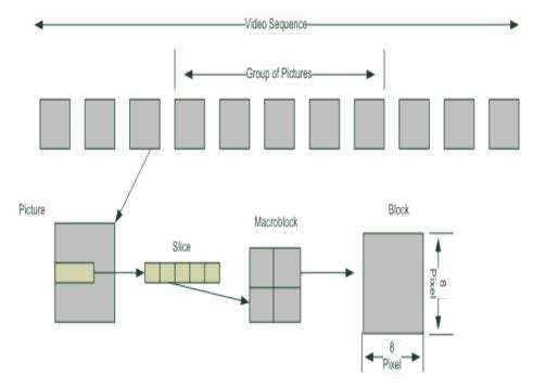
Figure 2.1: MPEG-2 Video Structure, adapted from [9]
