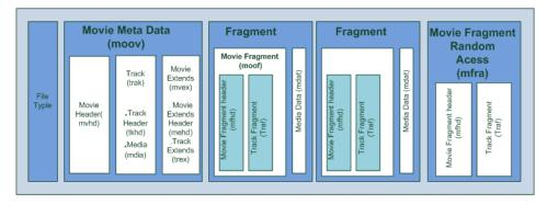
Figure 3.2: Disk File Format, adapted from [8]
