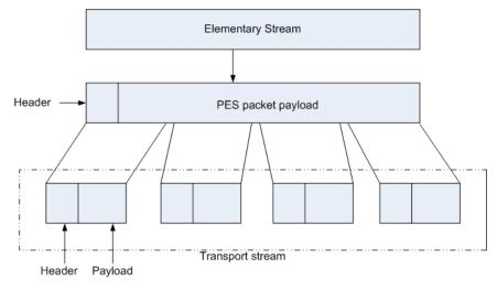
Figure 2.9: Transport Stream Generation, adapted from [19]
