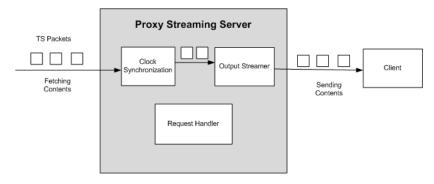
Figure 4.5: Output Streamer
