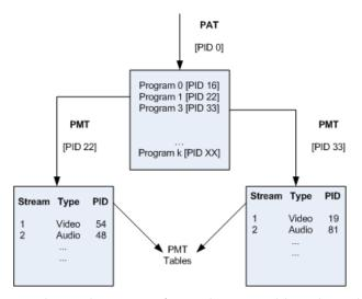
Figure 2.10: Relation between PAT and PMT table, adapted from [21]
