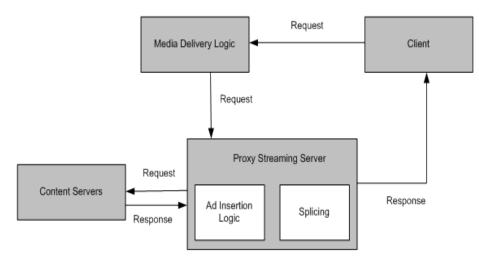
Figure 2.13: Overview showing the context of the splicing and advertisement insertion logic
