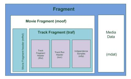
Figure 3.3: Wire file format, adapted from [8]
