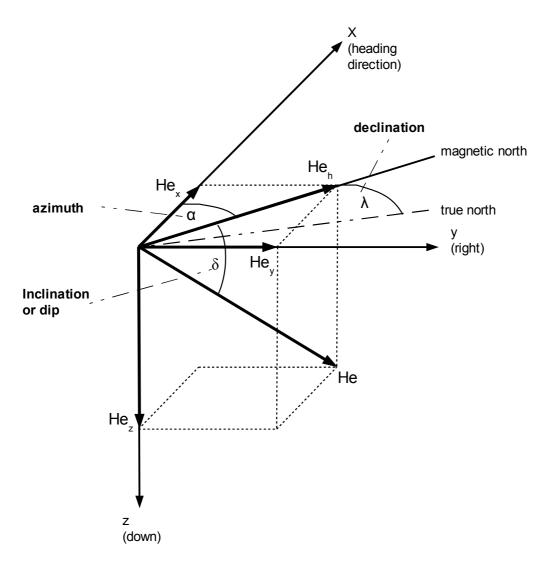
Figure 4. Earth magnetic field as a vector quantity
