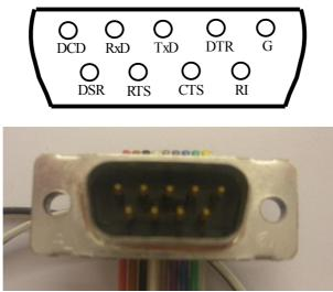
Figure 9. Male RS-232 pinout
