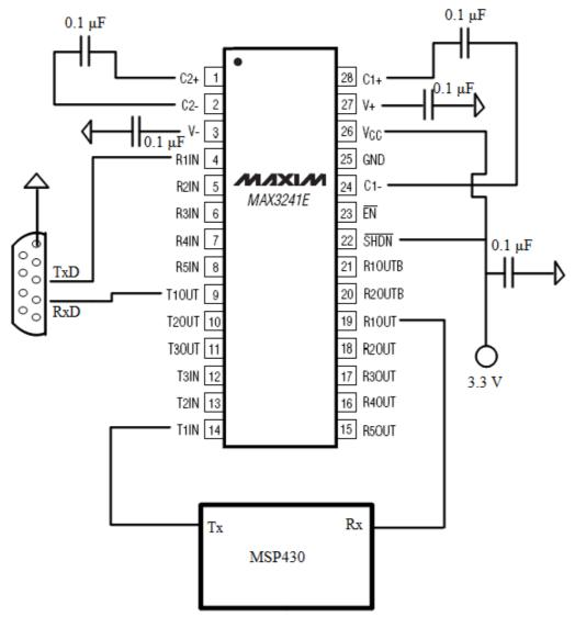
Figure 5. Level shifting schematics
