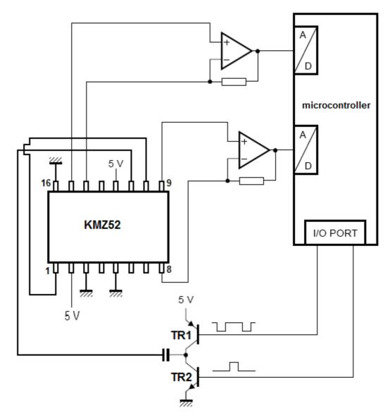
Figure 11. SCU with microcontroller
