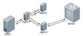
Figure 3.6. Diameter protocol error handling.
