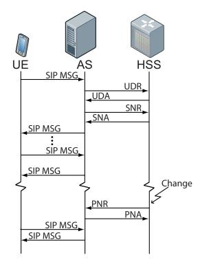
Figure 5.3. Example of message flow with AS caching and subscribing to user data to maintain cache coherence.
