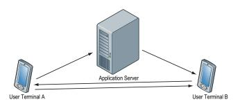
Figure 2.4. The AS handles the first message but then leaves the signaling path.
