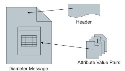
Figure 3.1. A Diameter message with header and Attribute Value Pairs
