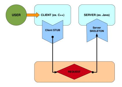
Figure 2.5. Client-server model in CORBA using stubs and skeletons
