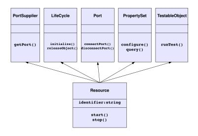
Figure 2.8. Resource Interface UML Diagram
