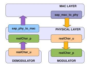
Figure 4.7. IDL interfaces for the physical layer
