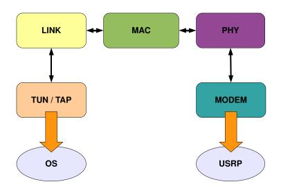
Figure 3.1. The waveform structure
