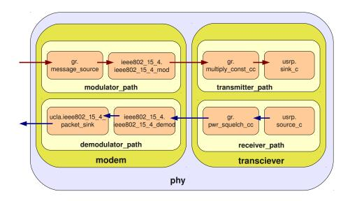
Figure 4.9. Physical layer structure in the GNU Radio IEEE 802.15.4 waveform
