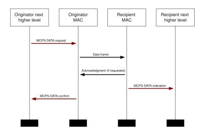
Figure 4.3. Message sequence chart describing the MAC data service (adapted from [24])
