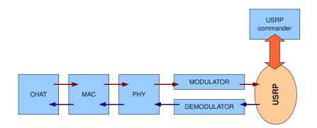
Figure 4.18. OSSIE waveform for the chat application
