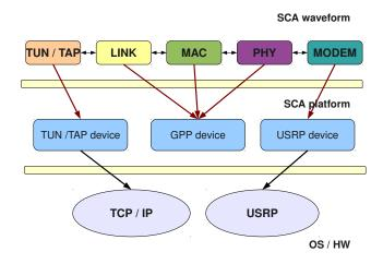
Figure 3.5. Waveform implementation using the SCA platform abstraction layer
