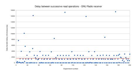
Figure 4.24. Data transfer delay for the USRP (GNU Radio implementation)
