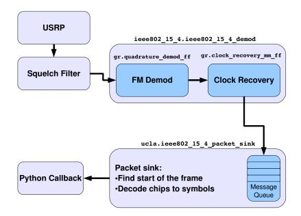
Figure 3.3. Block schema of the demodulator implemented in GNU Radio (adopted from [21])
