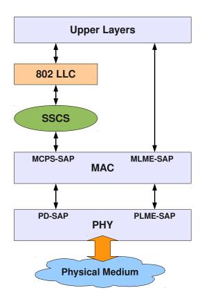
Figure 4.1. LR-WPAN device architecture (adapted from [24])
