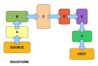
Figure 3.6. No blocks hierarchy in OSSIE waveforms
