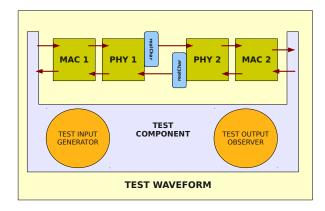
Figure 4.8. Waveform for testing the PHY layer component
