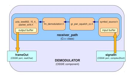
Figure 4.16. Internal structure of the DEMODULATOR component
