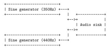
Figure 2.3. Flow graph of the GNU Radio dial tone example
