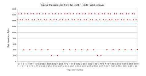
Figure 4.22. Data transfer size for the USRP (GNU Radio implementation)
