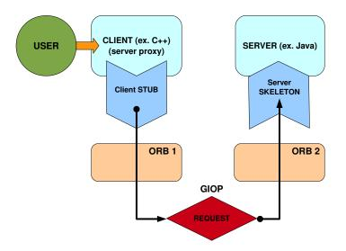
Figure 2.6. The inter-ORB communication using GIOP
