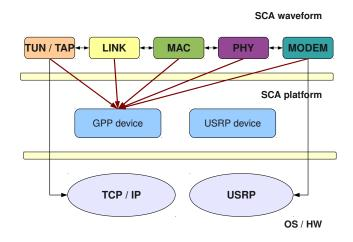
Figure 3.4. Waveform implementation without the SCA platform abstraction layer
