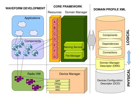
Figure 2.7. Abstraction layers in an SCA system
