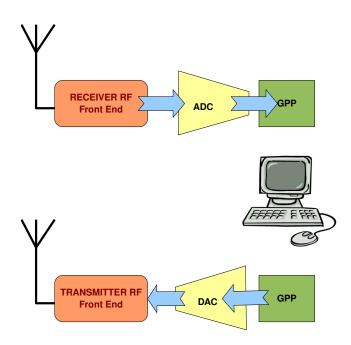
Figure 2.1. Ideal transmitter and receiver in SDR
