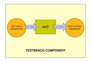
Figure 4.4. Testbench component for simulation of digital circuits in VHDL
