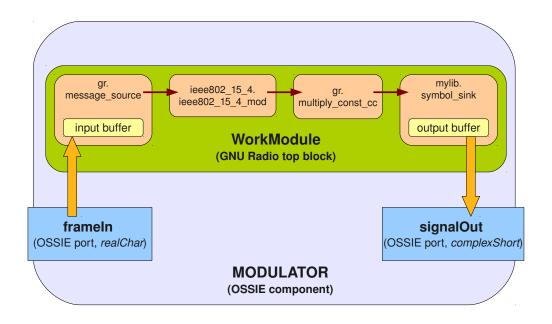
Figure 4.15. Internal structure of the MODULATOR component
