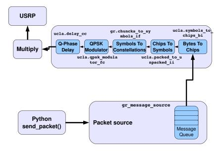
Figure 3.2. Block schema of the modulator implemented in GNU Radio (adopted from [21])
