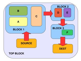
Figure 3.7. Blocks hierarchy in GNU Radio
