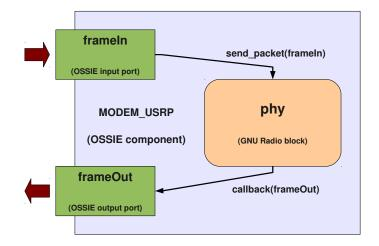
Figure 4.10. GNUARDIO\_MODEM component structure
