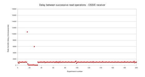
Figure 4.23. Data transfer delay for the USRP (OSSIE implementation)
