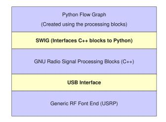
Figure 2.2. Block diagram of the GNU Radio architecture
