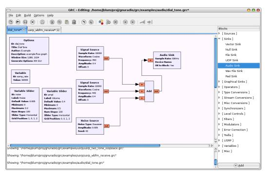
Figure 2.4. GNU Radio Companion (GRC), a tool for creating signal flow graphs and generating flow-graph source code
