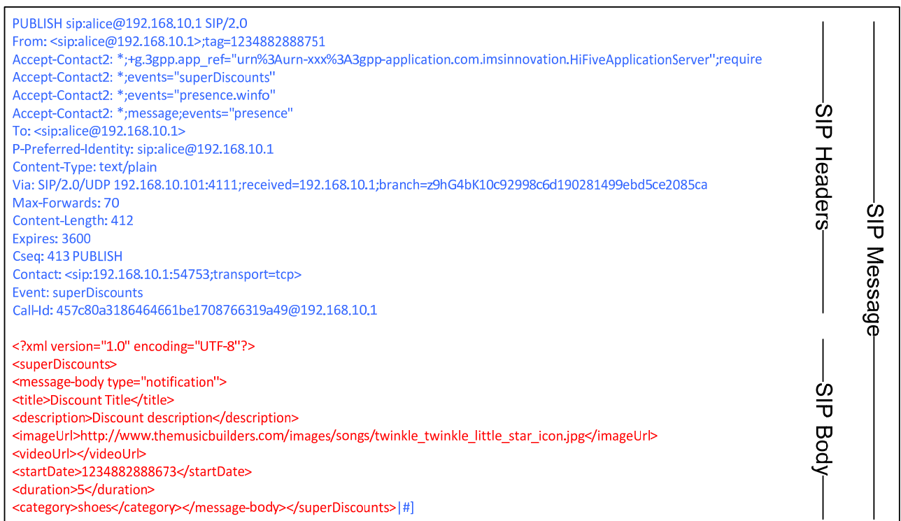
Figure 3-11: PUBLISH SIP message (discount upload)
