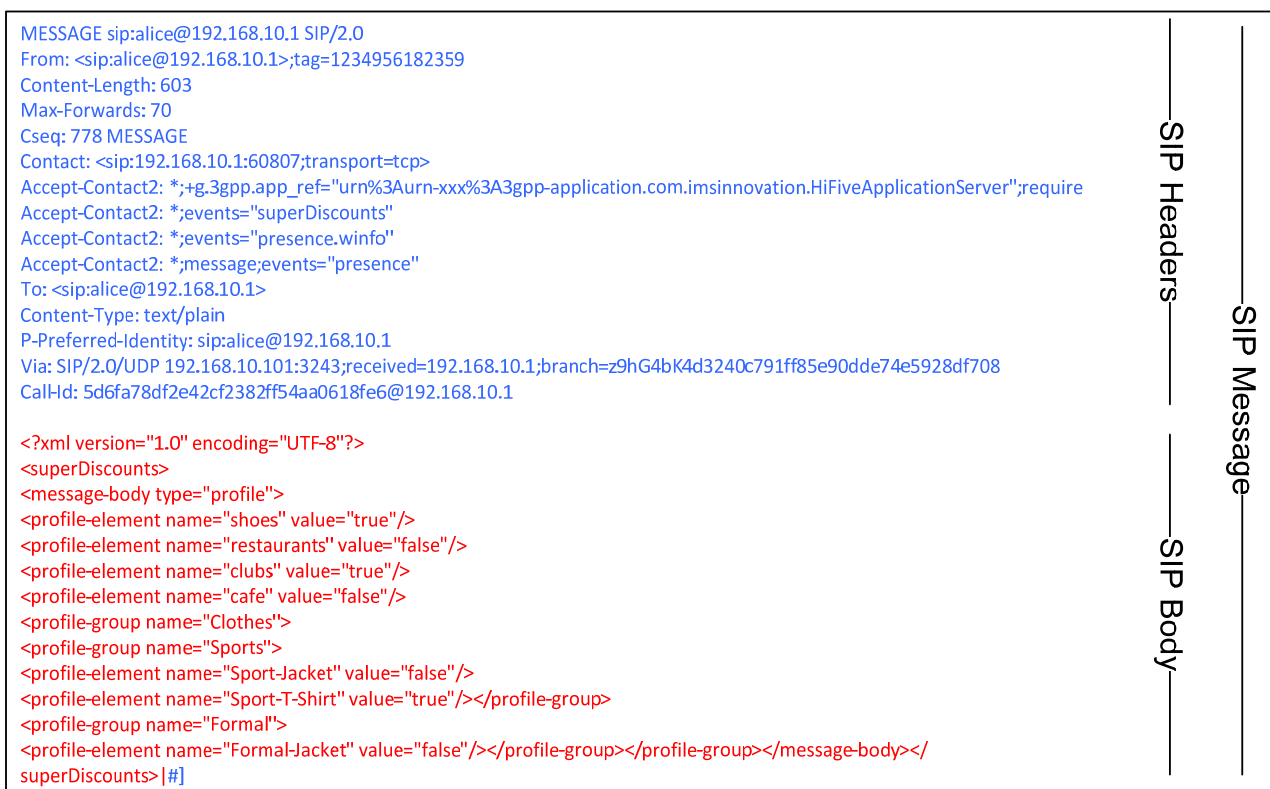
Figure 3-12: MESSAGE SIP message (profile upload)
