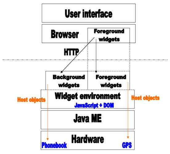
Figure 5: Hierarchical architecture diagram.
