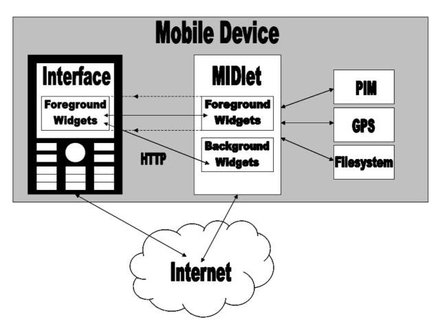
Figure 3: Architecture of the prototype implementation
