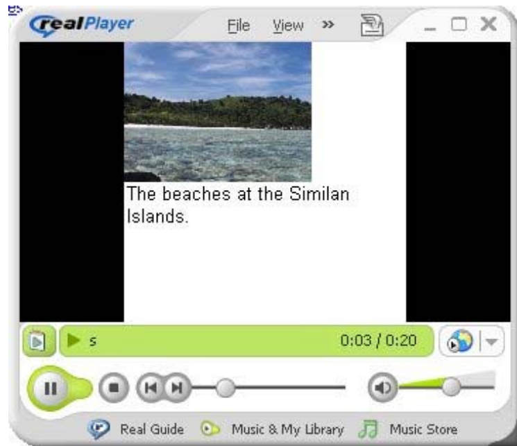
Figure 1. MMS SMIL displayed in RealNetworks' RealPlayer. All elements are displayed, but the display area is not fully utilized.
