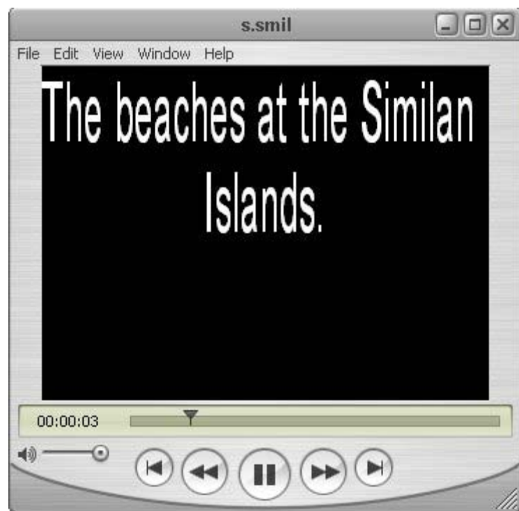
Figure 2. MMS SMIL displayed in Apple's QuickTime. Only the text appears and it does so both enlarged and with inverted colors.
