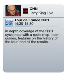
Figure 4.8. View D3. This is the full screen equivalent of the A3 view. You enter this view by pressing the hash key in the A3 view or by navigating here from the D2 view. If the program description text is too long, a scrollbar will appear, which you can scroll by navigating up or down. Navigate left to go back to the D2 view or press the hash key to go to the A1 view.
