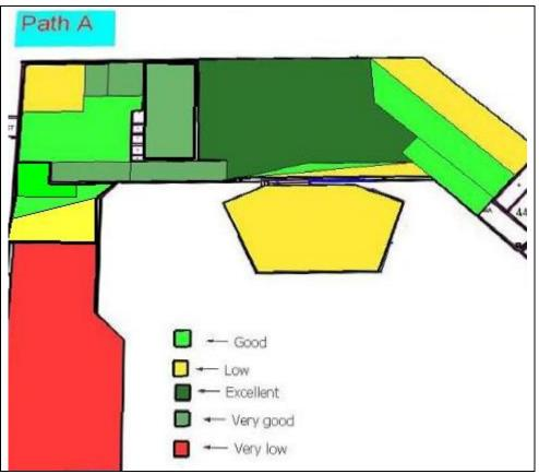
Figure 22. Signal distribution of access point 2 in the path A.
