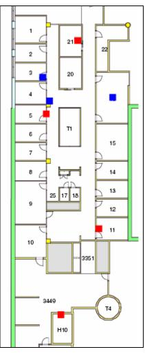
Figure 26. Blue rectangles are places where Open network were scanned and red rectangles are place of APs.
