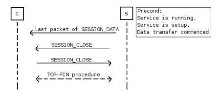
Figure 20: Disconnection procedure between Client and Server
