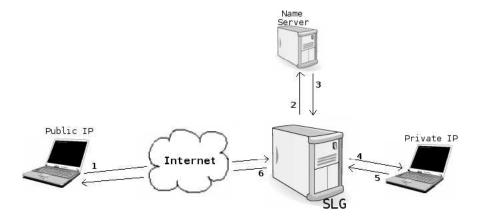
Figure 6: Public to Private network through SLG in setup mode
