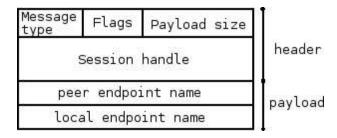
Figure 9: Control Packet with header and payload
