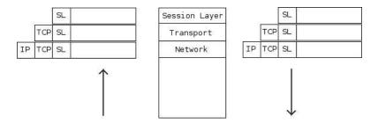
Figure 7: Unpacking and re-packing a packet
