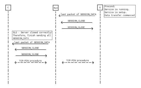
Figure 19: Disconnection procedure between Client and Server through SLG
