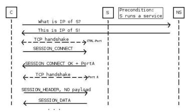
Figure 16: Setup procedure between Client and Server
