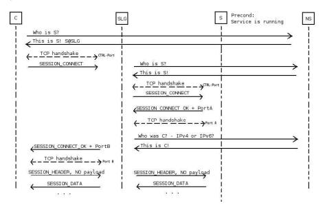
Figure 15: Setup procedure between Client and Server through SLG
