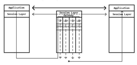
Figure 5: Schematical view of the communication process between two peers through the SLG
