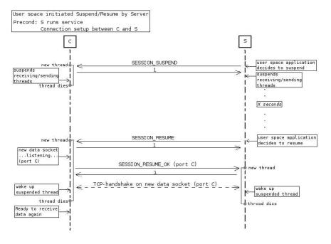
Figure 18: Suspend and resume procedure between Client and Server
