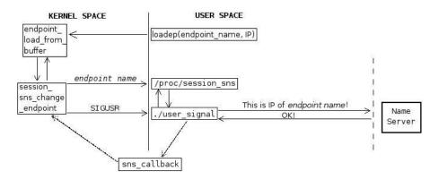
Figure 22: Endpoint update signaling
