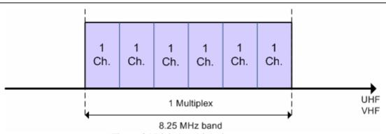
Figure 4.1 Digital multiplexing structure
