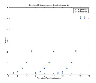
Figure 27: Logger Simulation vs. Experiment with reading interval 3s
