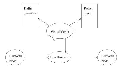
Figure 23: Virtual Merlin's NS2-UCBT connection
