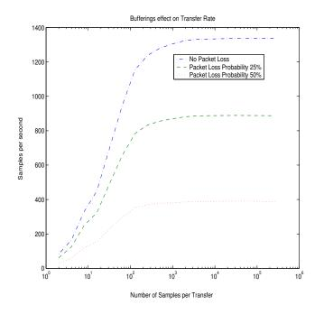
Figure 48: Samples per Second with Different Buffer sizes
