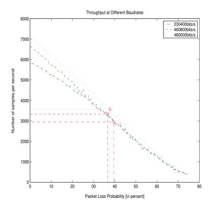
Figure 52: Samples Per Second with Higher Baudrates
