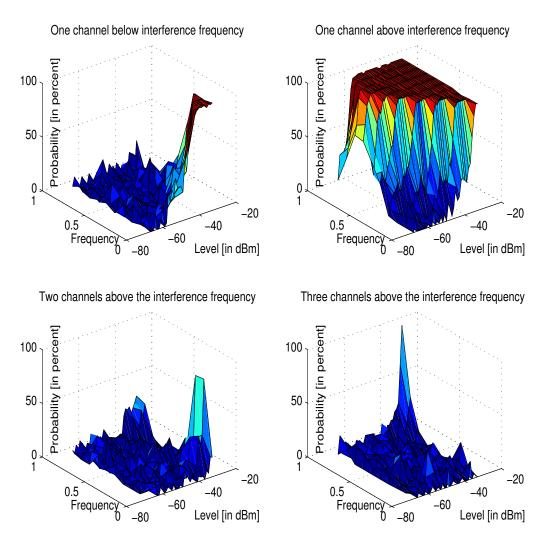
Figure 35: Packet Loss Probability for adjacent channels ch - 1, ch + 1, ch + 2 and ch + 3
