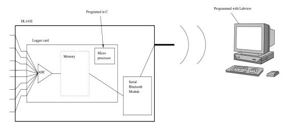
Figure 16: The DL141E structure
