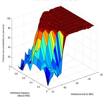
Packet loss probability at different interference frequency offsets
