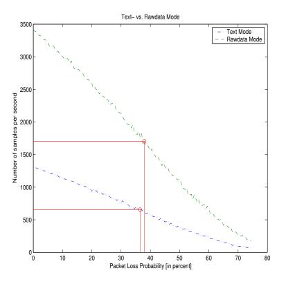
Figure 50: Samples Per Second with Text- vs. Rawdata Mode
