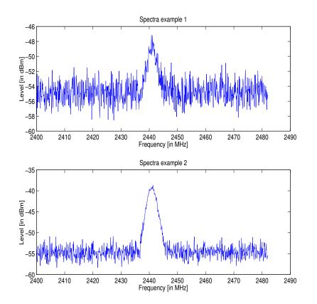
Figure 31: Two Interference Spectra Examples
