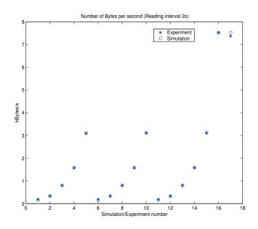
Figure 26: Logger Simulation vs. Experiment with reading interval 2s
