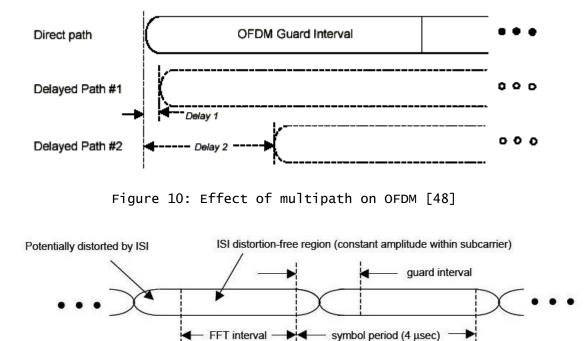
Figure 11: OFDM Symbol Contains a Guard Interval [48]
