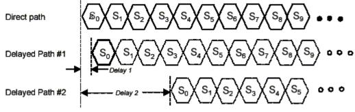
Figure 9: effect of multipath on CCK [48]
