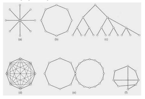
Figure 2-3 Traditional topologies for a point-to-point network
