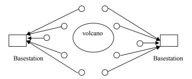
Figure 2-6 A tree topology volcano sensor network
