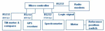
Figure 1-2 System diagram
