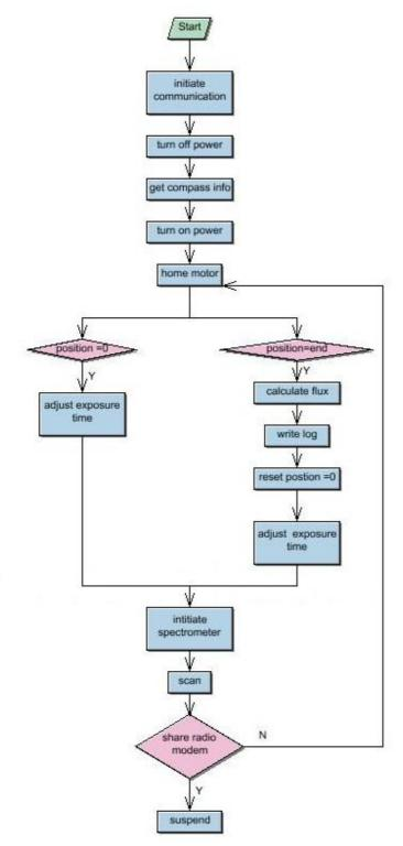
Figure 4-3 Flow chart of the remote control program
