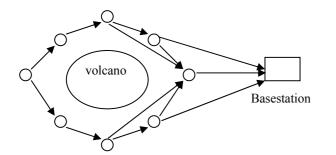
Figure 2-5 An example topology for a volcano sensor network
