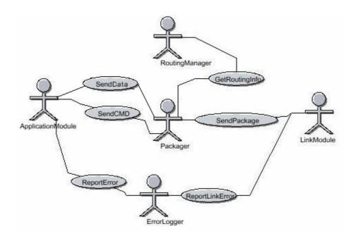
Figure 3-3 Network module of basestation
