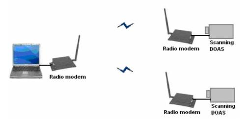
Figure 4-2 Radio network solution for volcano monitoring sensor network
