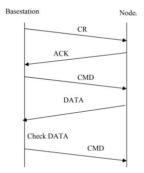
Figure 2-9 (e) Transmission scenarios - Data is incorrect
