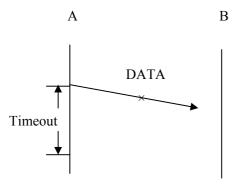
Figure 2-8 (b) Error control in data link layer - DATA lost
