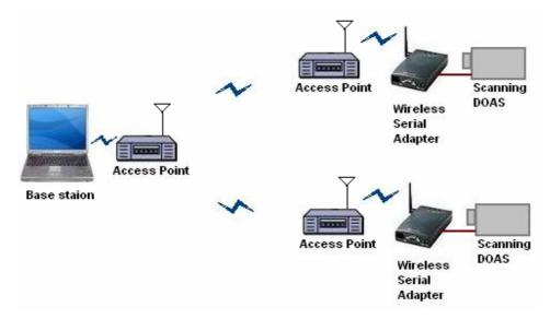
Figure 4-1 WLAN solution for volcano monitoring sensor network
