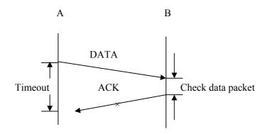
Figure 2-8 (c) Error control in data link layer - ACK lost
