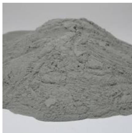
Figure 4: Very fine aluminium powder which can be used for sintering. [12]
