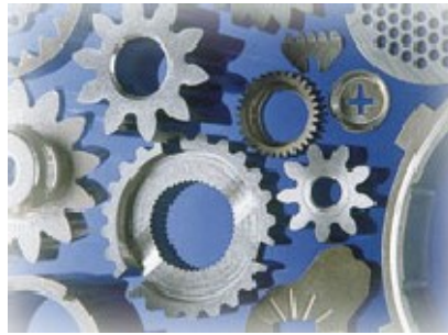
Figure 6: Various gears made through sintering. [20]
