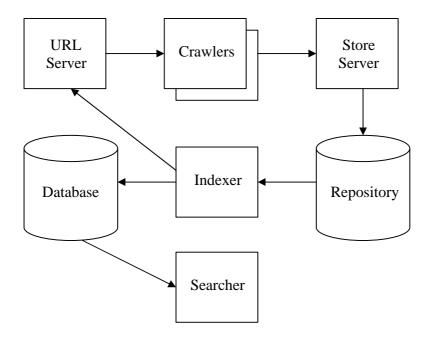
Figure 1. High level system architecture of a typical search engine.
