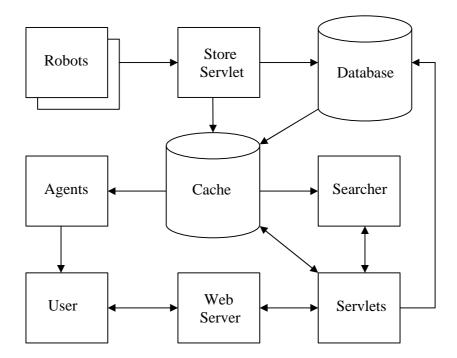
Figure 2. High level system architecture of the prototype search engine.
