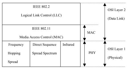
Figure 1: IEEE 802.11 standards mapped to the OSI reference model
