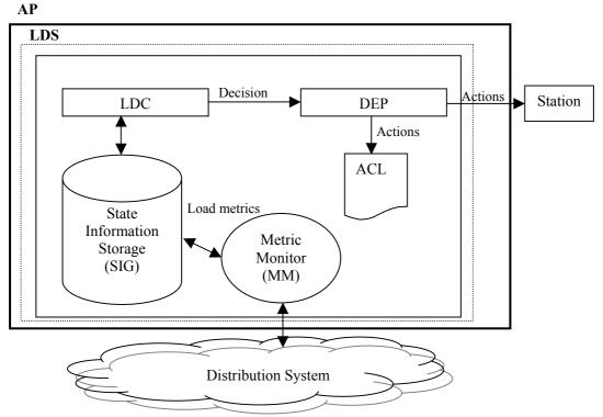
Figure 8: Load Distribution System components
