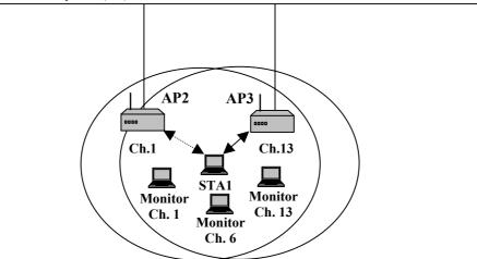
Figure 13: Test-bed configuration to measure handover time
