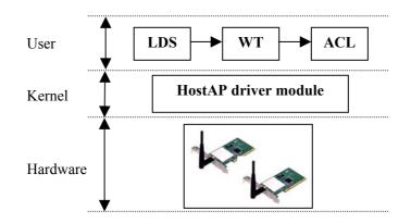
Figure 12: Position of the LDS in the prototype
