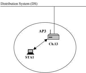
Figure 18: Test-bed configuration to test the sampling time of the metric monitor
