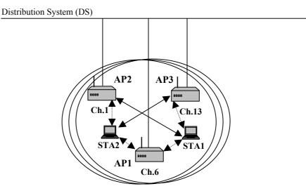
Figure 30: Test-bed configuration to test the transfer policy performance
