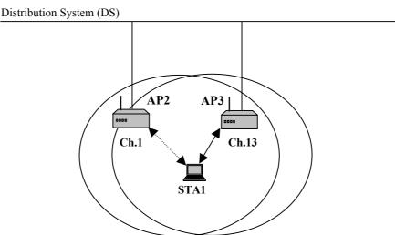
Figure 20: Test-bed configuration to test the reactivity of the LDA
