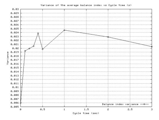
Figure 22: Variance of the average balance index for values of the CT = 0 (without LDS), 0.1 s, 0.2 s, 0.3 s, 0.4 s, 0.5 s, 1 s, 2 s and 3 s
