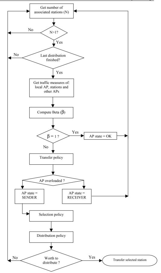
Figure 9: Block diagram of the load distribution algorithm (LDA)
