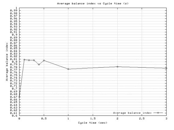
Figure 21: Average balance index ( $\beta_{avg}$ ) for values of the CT = 0 (without LDS), 0.1 s, 0.2 s, 0.3 s, 0.4 s, 0.5 s, 1 s, 2 s and 3 s
