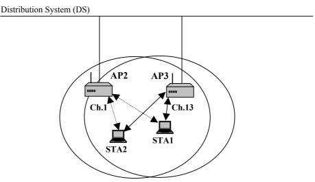
Figure 27: Test-bed configuration to measure packet delay
