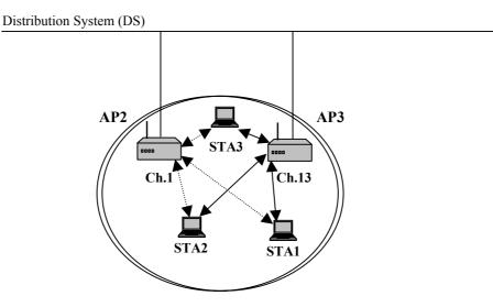
Figure 33: Test-bed configuration to determine the distribution time
