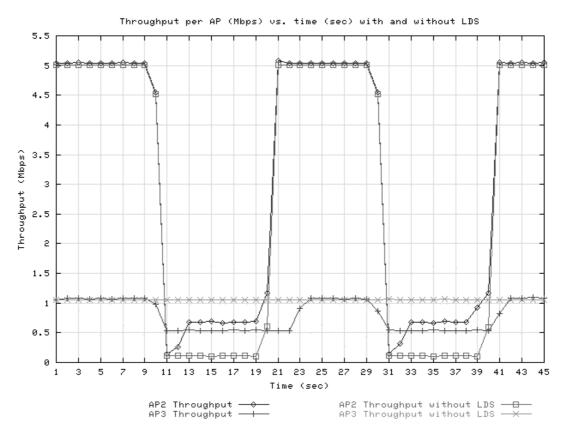
Figure 26: Throughput of AP2 and AP3 with and without load distribution
