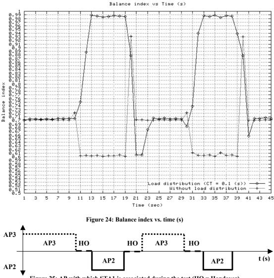
Figure 25: AP with which STA1 is associated during the test (HO = Handover)
