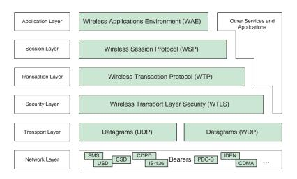
Figure 3.2: The WAP stack reference model [234]
