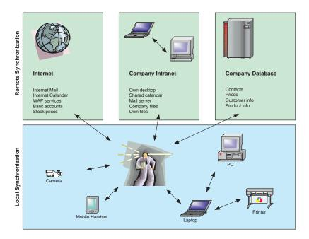
Figure 3.6: Scenarios for synchronizing with SyncML
