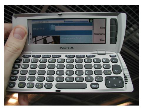
Figure 2.8: The Nokia 9210 Communicator with EPOC OS
