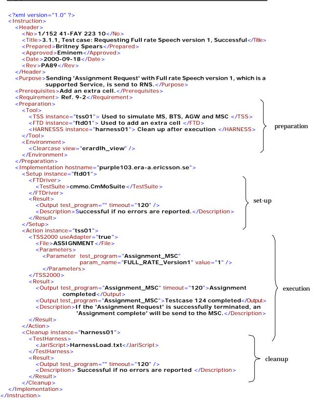
Figure B - 2: An example of a test case document.
