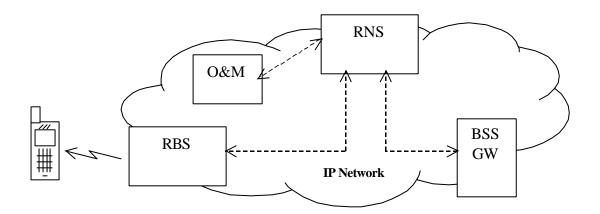
Figure 2 - 1: Illustrating the different nodes of the complete IP-BSS system. The separate parts are developed by different units within Ericsson, in parallel. The main focus of this project is the verification of functionality in the Radio network Server (RNS) node.
