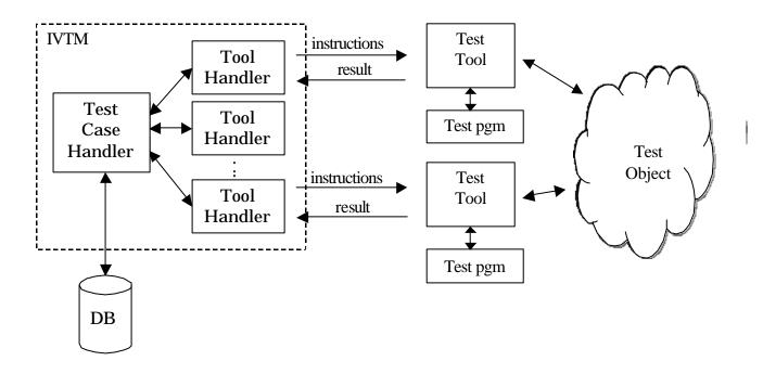
Figure 4 - 2: illustrating the role of the tool handlers in the system model. The test case handler is connected to a database or file system where test case documents and reports are stored
