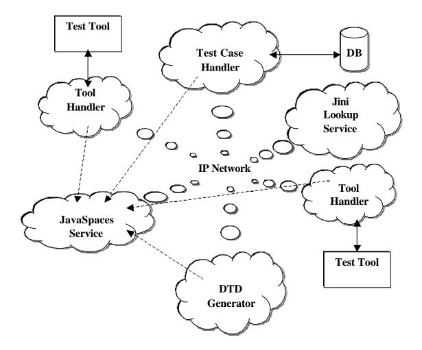
Figure 5 – 1: The different system components does not know neither what other components are running on the network nor their location. Still they can interact through the common JavaSpaces Service. The JavaSpace is located through the Jini Lookup Service, which is located by sending a multicast message and then wait for a reply.
