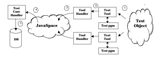
Figure 5 – 5: flow of events when reporting result from test case.
