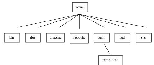
Figure B – 1: Illustrating the directory structure of the IVTM.
