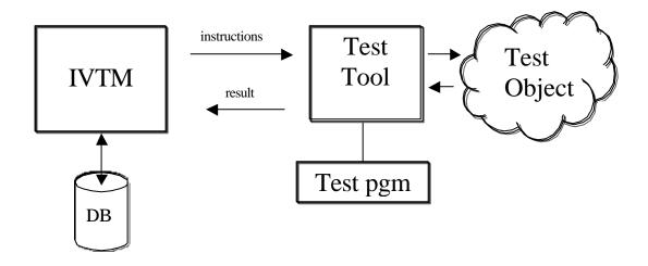
Figure 4 - 1: illustrating the relationship between test tool, test program, test object and the test model.
