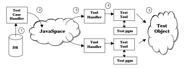
Figure 5 – 4: flow of events when executing test cases.
