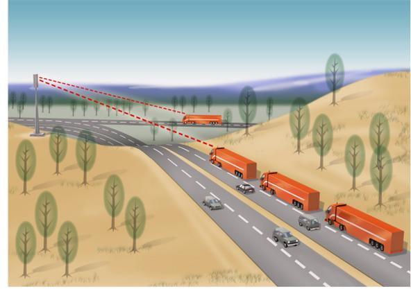
**Fig. 11.** Automatic control of a merging maneuver, where a single vehicle is about to merge with a three-vehicle platoon after a road intersection. The operation is supported by vehicle-to-infrastructure communication.
