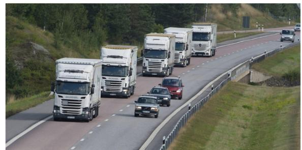
Fig. 2. A platoon of five trucks driving close together to save fuel.
