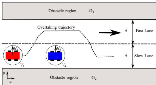
Fig. 1. Scenario where an automated vehicle  $V_1$  is overtaking a human-driven vehicle  $V_2$  on a road with two lanes.
