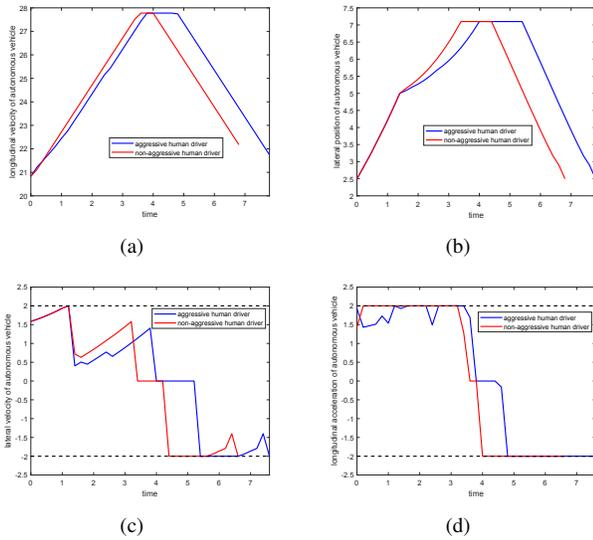
Fig. 4. State trajectories and control inputs of the automated vehicle under Algorithm 1 for the aggressive human driver and Algorithm 2 for the non-aggressive human driver: (a) longitudinal velocities; (b) lateral positions; (c) lateral velocities; (d) longitudinal acceleration.
