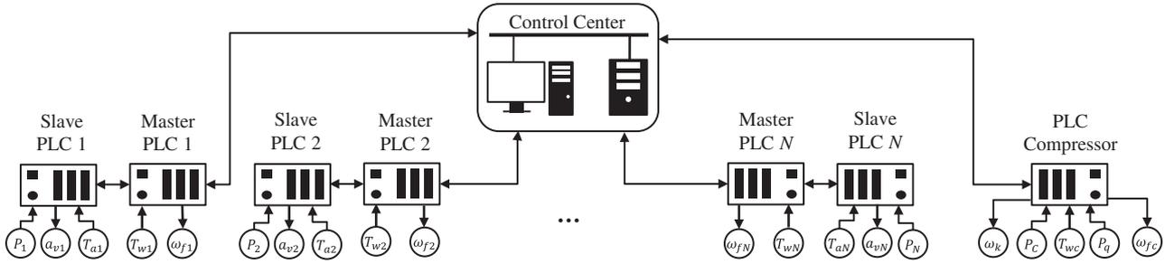
**FIGURE 5** Cyber infrastructure of the variable refrigerant flow control system. PLC, programmable logic controller
