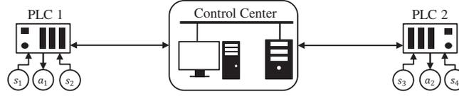
**FIGURE 2** Example of an industrial control system consisting of the control center, two programmable logic controllers (PLC 1 and PLC 2), two actuators ( $a_1, a_2$ ), and four sensors ( $s_1, s_2, s_3, s_4$ )
