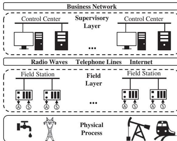
**FIGURE 1** Common architecture of an industrial control system. The physical process is controlled through the field layer, which consists of control devices, sensors, and actuators. The supervisory layer is used for monitoring and control of the field layer, consists of ordinary IT equipment, and is often connected to other networks
