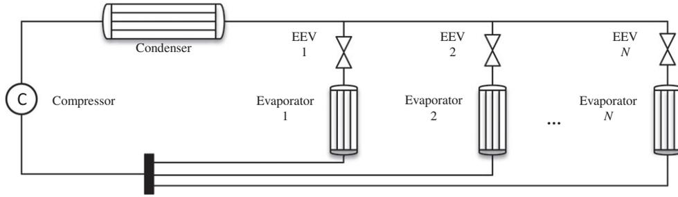
**FIGURE 4** Physical infrastructure of the variable refrigerant flow control system. EEV, electronic expansion valve
