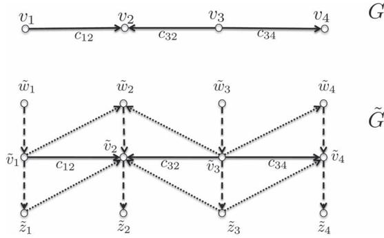
Fig. 3. Representation of the auxiliary graph  $\tilde{G}$  associated to the graph  $G$ . The dotted diagonal edges all have the same weight  $C > \max p_i$ . The vertical dashed edges linking  $\tilde{w}_i$  to  $\tilde{v}_i$  and  $\tilde{v}_i$  to  $\tilde{z}_i$  have weight  $p_i$ .
