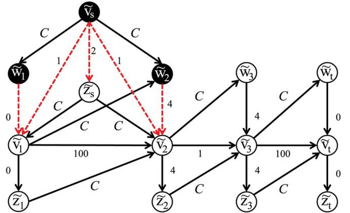
Fig. 5. Solving the standard  $\text{Min Cut}$  problem in the auxiliary graph corresponding to the instance in Fig. 4 (the irrelevant node  $w_s$  is not shown).  $C$  is a large scalar constant defined in the auxiliary graph construction procedure in Section V-A. The black nodes form the optimal source set (in the auxiliary graph), and the dotted red edges are cut. The optimal objective value is 8.
