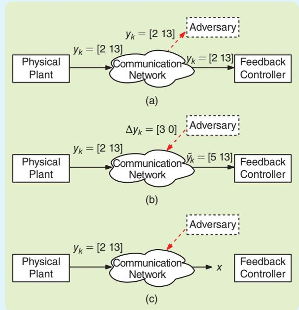
**FIGURE S1** Cyberattacks on a communication network: (a) data confidentiality violation by a disclosure attack, (b) data integrity violation by a false-data injection attack, and (c) data availability violation by a denial-of-service attack.
