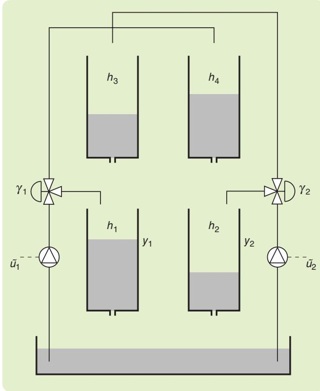
**FIGURE 14** A schematic of the quadruple-tank process [66]. The water pump to the left is controlled by the signal  $\tilde{u}_1$ , while the pump to the right is controlled through  $\tilde{u}_2$ . The left pump forces water into tanks 1 and 4, where the fraction of water flowing into each tank is determined by the valve position  $\gamma_1$ . Similarly, the fraction of water pumped to tanks 2 and 3 by the right-hand-side pump depends on  $\gamma_2$ .
