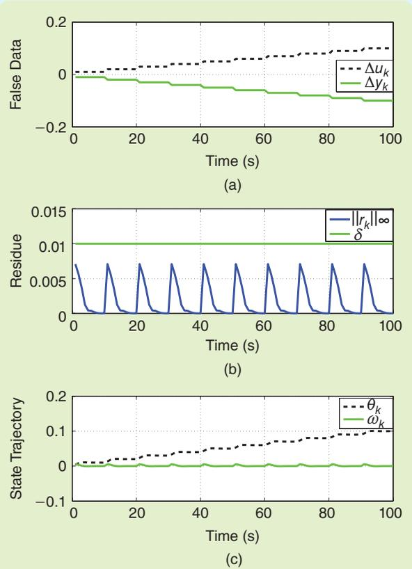
**FIGURE S2** Simulation results from the attack policy (S2) with  $N = 10$ ,  $\lambda = 1$ , and  $g = [-0.01 \ 0.01]^T$ . Plot (c) depicts the state trajectory under attack, the injected false-data is shown in (a), and (b) illustrates the corresponding residue signal and detection threshold.
