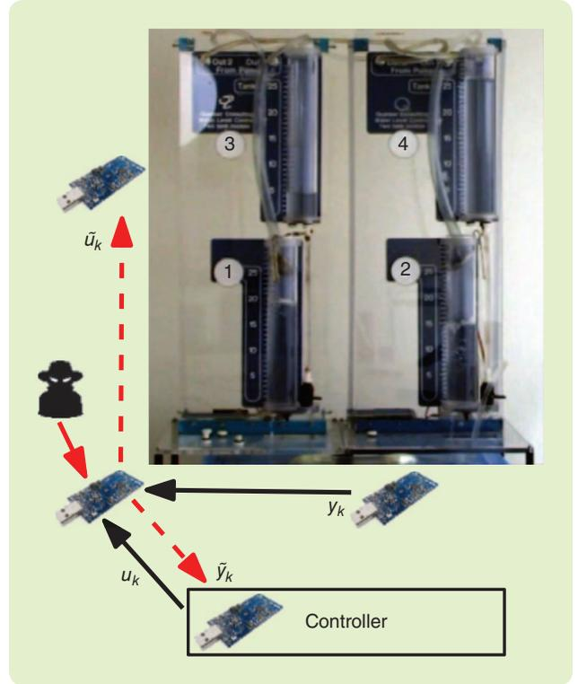
**FIGURE 15** A schematic diagram of the test bed with the quadruple-tank process and a multihop communication network. The controller, sensors, and actuators communicate using a wireless network that has one relay node. The adversary is able to compromise the relay node and therefore has access to the control and measurement channels.
