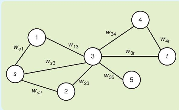
**FIGURE S3** An instance of a minimum cut problem is defined on an undirected graph with nonnegative edge weights. The nodes  $s$  and  $t$  denote the source and sink, respectively. For an edge connecting node  $i$  and node  $j$ , the quantity  $w_{ij} \geq 0$  is the corresponding edge weight.
