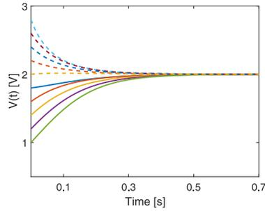
Fig. 4. Nodal voltages with controllers (8). Matrix  $\Psi^\ell$  is Metzler and Hurwitz, and the network is cooperative.
