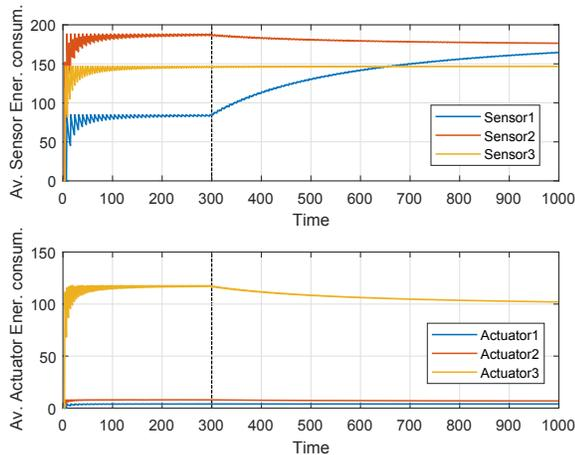
Fig. 7. Averaged energy consumption for sensor and actuator communication
