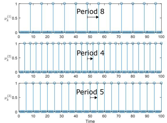
Fig. 5. Optimal schedules of three loops
