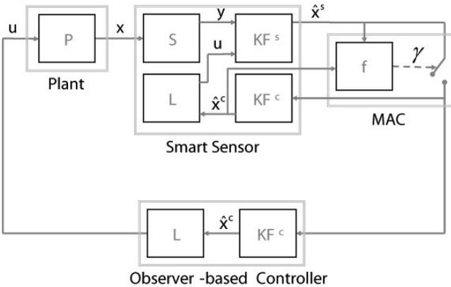
Fig. 1. The system architecture (dual predictor) with MAC
