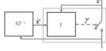
Fig. 4. An adaptive medium access controller
