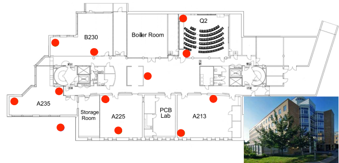
Fig. 13. HVAC testbed at the second floor of the Q-building at KTH. Each of the five rooms considered contain sensors and actuators used for HVAC control. Additional sensors are located in the corridor and outside of the building.
