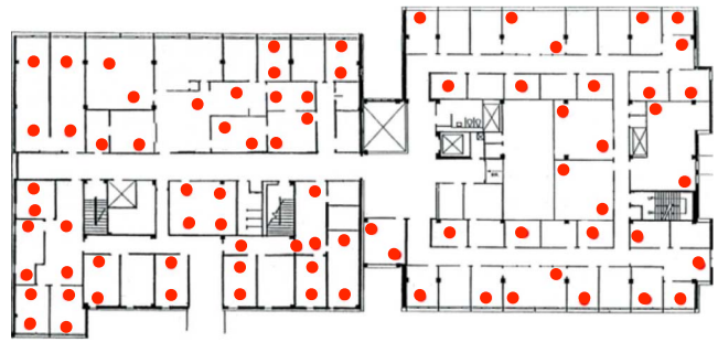
Fig. 12. WSN testbed in Bryan Hall and Jolley Hall of Washington University in St. Louis.
