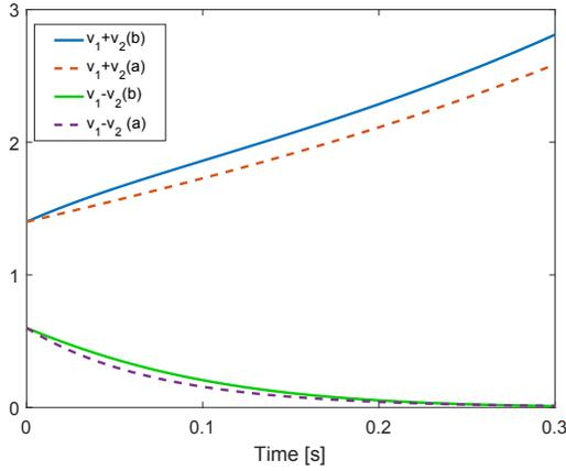
Fig. 2. The growth of the sum and the decay of the relative voltages for a two node graph for constant (a) and voltage-dependent(b) networks.
