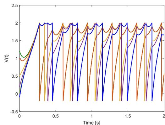
Fig. 6. Voltage trajectories for the network with constant and common coupling with  $g = 2.8$ .
