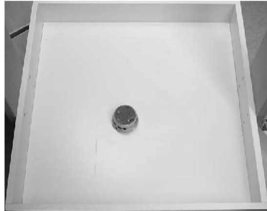
Figure 9: Experimental setup for evaluation of the area coverage robot.
