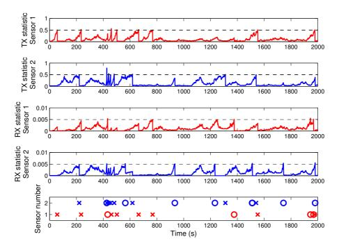
Fig. 3. Transmission and reception statistics for wireless sensor 1 and 2 in transient conditions; Transmissions is characterized by a cross (×) and receptions by a circle ( $\circ$ ). Tank 1 and tank 2 levels are shifted at time t = 400 s and at t = 420 s, sensor 1 avoids transmission since it receives information from the central estimator. The listening benefit is observed also for sensor 2 at time t = 934 s and t = 1980 s and for sensor 1 again at t = 1374 s.
