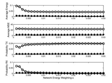
Fig. 5. Steady-state condition statistics in terms of average energy, MSE and probability of transmissions (TX) and reception (RX) for the case of: No tank level shift (Star ( $\star$ )) and with periodic tank level shifting every 100 s (Circle ( $\circ$ )).
