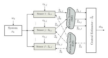
Fig. 1. Distributed event-triggered estimation system architecture.
