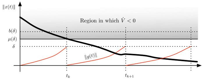
**Fig. 1.** The proposed event-triggered sampler. Every time the error function  $\|g(t)\|$  hits the threshold  $\delta$ , then the system is sampled again, and the error is reset. By doing that the Lyapunov derivative is strictly negative in the region  $\|x\| > \mu(\delta)$ , and then the trajectories must converge into an invariant set.
