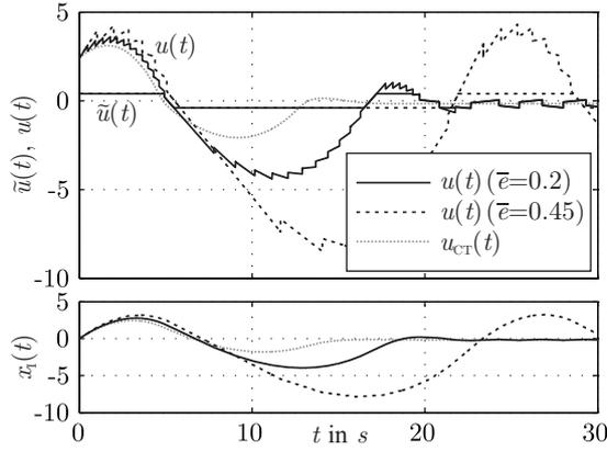
Fig. 4. Control inputs  $\tilde{u}(t)$ ,  $u(t)$  and integrator state  $x_I(t)$  for the continuous-time control loop (grey dotted curves), the event-triggered control loop with  $\bar{e} = 0.2$  (black solid curves) and the event-triggered control loop with  $\bar{e} = 0.45$  (black dashed curves)
