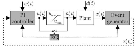
Fig. 7. Event-triggered anti-windup scheme (ETAW)
