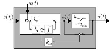
Fig. 6. Smart actuator including the controller and a dynamic anti-windup scheme (CTAW)
