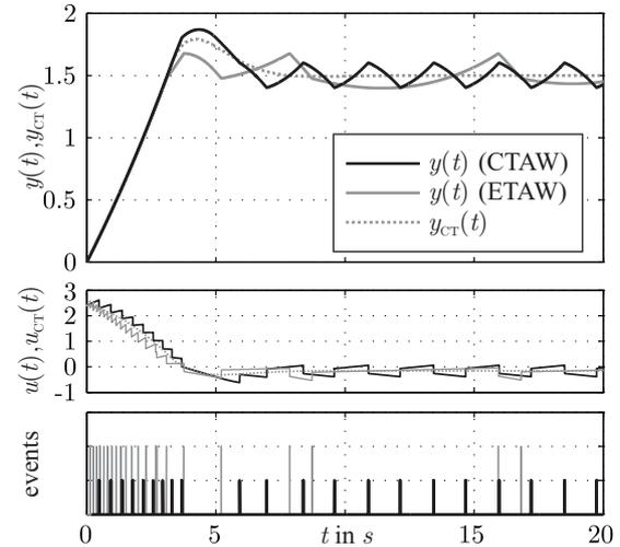
Fig. 8. Behavior of the continuous-time control loop and the event-triggered control loop using anti-windup techniques
