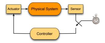
In time-triggered control the sensing, control, and actuation are driven by a clock.
