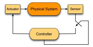
In self-triggered control, the current state is used not only to compute the input to the system, but also the next time the control law should be recomputed;
