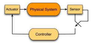
This can be regarded as introducing *feedback* in the sampling process! Event-triggered control requires the constant monitoring of the state to determine current performance. In self-triggered control, the current state is used not only to compute the input to the system, but also the next time the control law should be recomputed;
