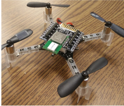
Fig. 10. CrazyFlye 2.0 quadrotor helicopter with UWB expansion.
